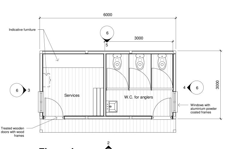
TEMPORARY STRUCTURE (Pre-fabricated for minimal disruption to the area during installation)
